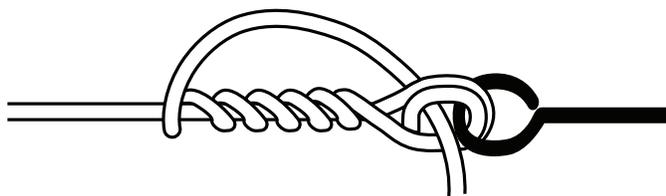
3. Thread the tag end back between the eye and the coils as shown.
