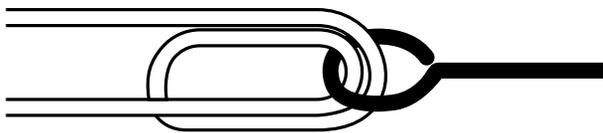
1. Run the end of the line through eye of hook and lure and double back through the eye a second time.
